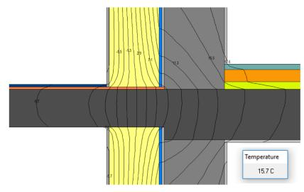
The minimal interior surface temperature is determined through another simulation. This one will be identical to the first one, except from the fact that the surface internal resistance is 0.25 (m<sup>2</sup>K)/W for all the internal surfaces.
