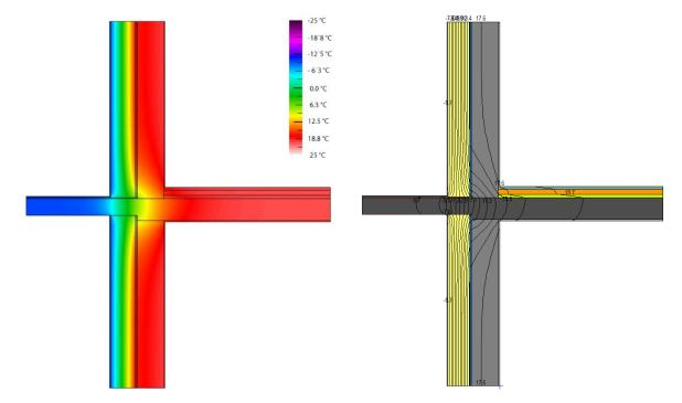
5. A drawing with isothermal lines as output from the software used
