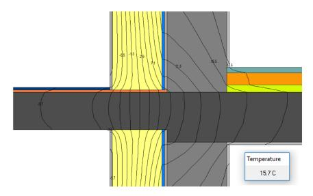
The minimal interior surface temperature is determined through another simulation. This one will be identical to the first one, except from the fact that the surface internal resistance is 0.25 (mK)/W for all the internal surfaces.
