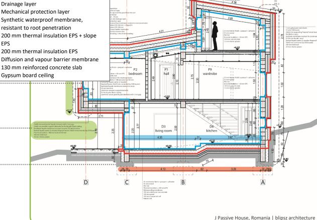
Graphic identification and external dimensions of the thermal envelope
