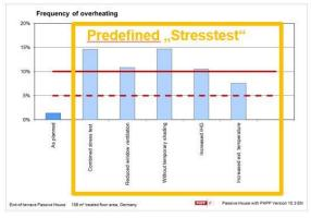
Stress test for summer comfort: the PHPP planning tool shows the frequency of overheating that would occur in various scenarios. Plans can be adjusted accordingly. © Passive House Institute
