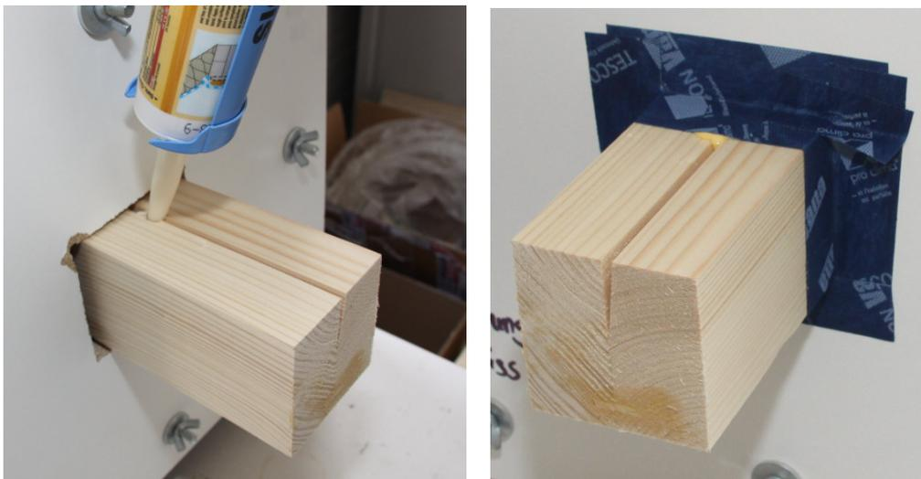
**Figure 25:** A hole is drilled in the crack at the later sealing level and filled with sealant (solution for drilled hole with sealant, left). The beam is then sealed with the cover using adhesive tape (right)
