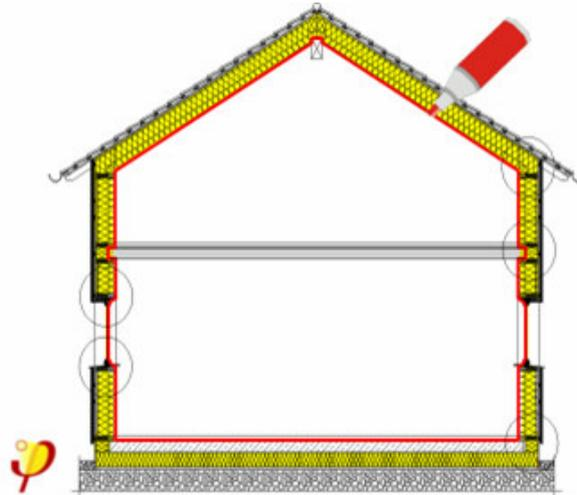
**Figure 3:** In the sectional drawing the airtight layer can be outlined without having to take the pencil off the paper ("pencil rule") (Source: PHI)
