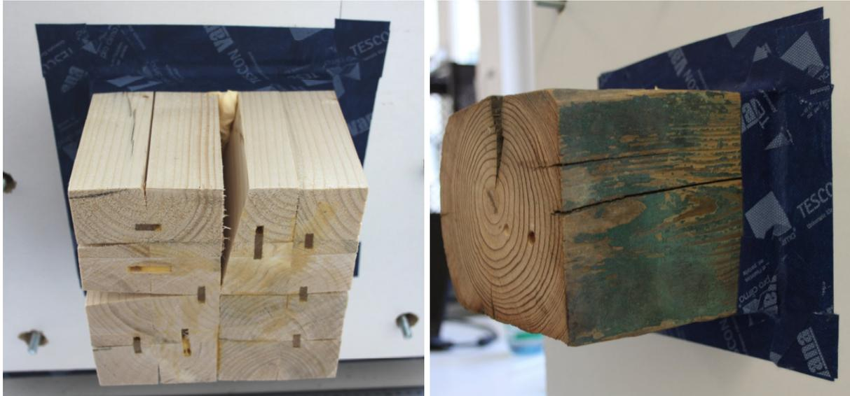
**Figure 33: Sealed "large" sample beam (left) and "old" or "real" beam (right)**
