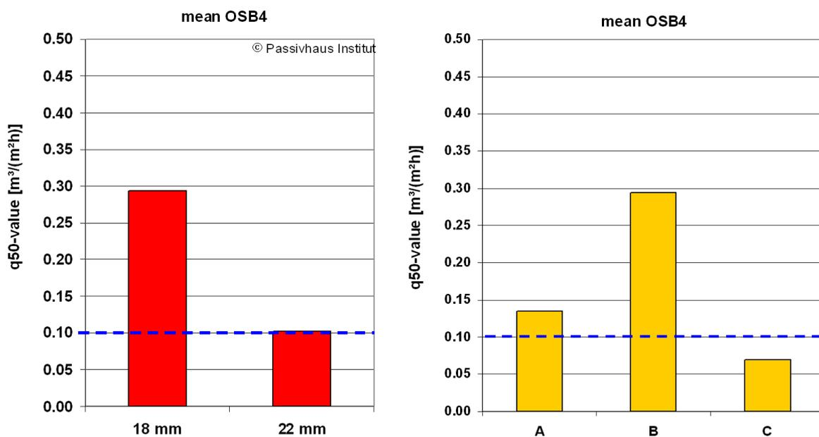
**Figure 39:** Average values of the Type 4 OSBs shown in Figure 37 according to board thickness (left) and according to manufacturers (right). Blue line: target value  $q_{50} = 0.1 \text{ m}^3/(\text{m}^2\text{h})$ .
