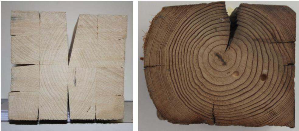
**Figure 13:** Cut surface of the large sample beam (ca. 16 mm x 15 mm) and of the old beam (ca. 120 mm x 145 mm)
