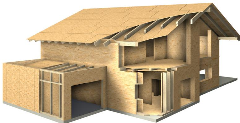
**Figure 35: An "extreme case": a single-family home built entirely with wooden OSBs (Picture: Norbord)**
