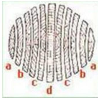
**Figure 8: Anisotropic shrinkage and expansion of wood (Source: [Hol])**
