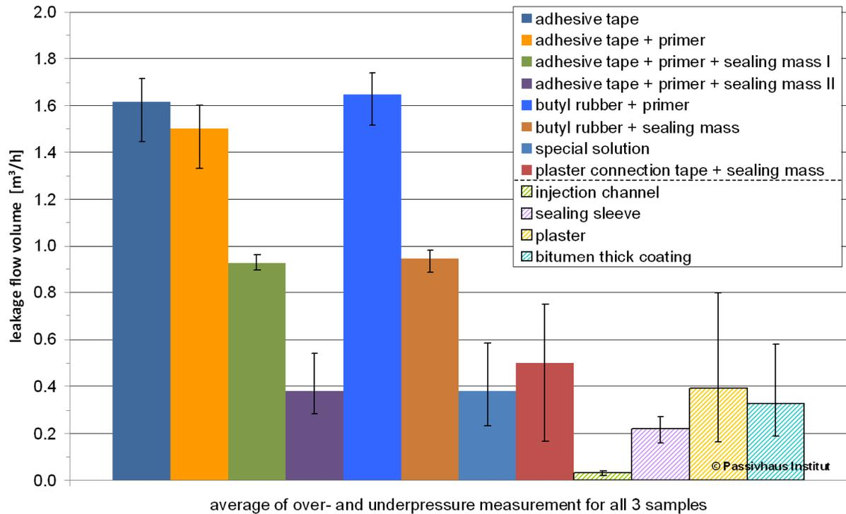
**Figure 32:** Comparison of the leakage flows in the measurements carried out, standardised for a differential pressure of 50 Pa (average value of the excess and negative pressure measurement for the three samples respectively). The thin black line shows the respective minimum and maximum value that was measured.
