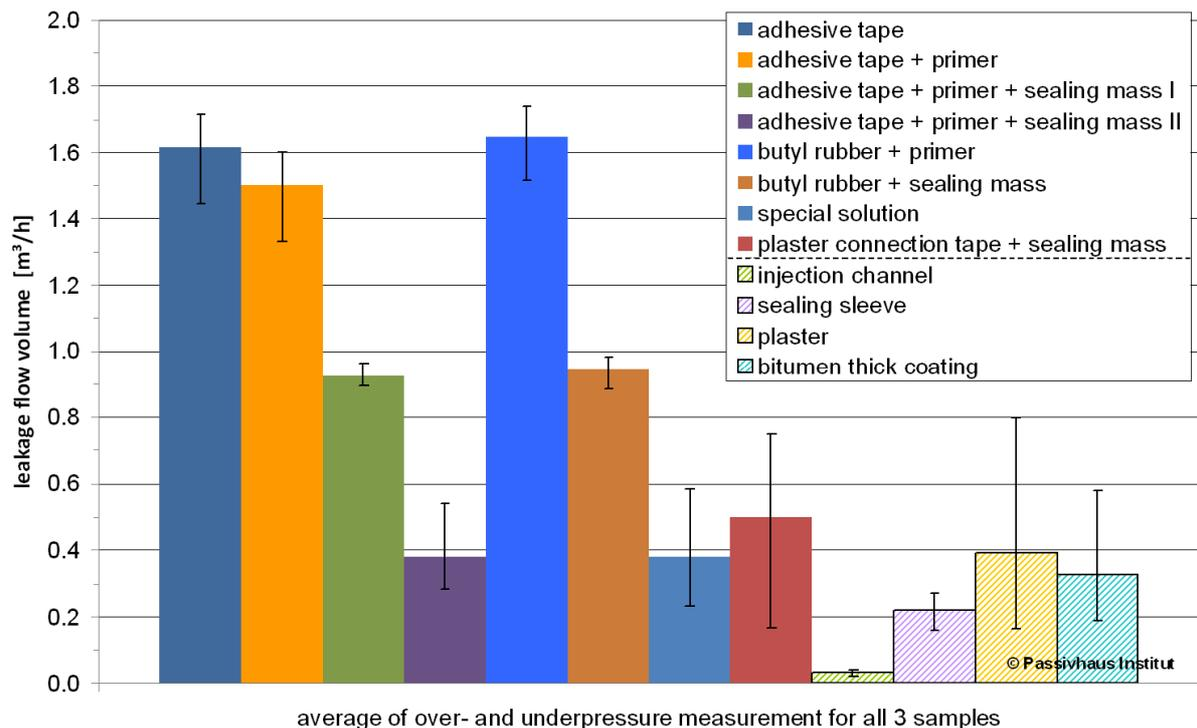
**Figure 1:** Comparison of the leakage flows during the measurements, standardised for a pressure difference of 50 Pa (average value of the excess and negative pressure measurement of the three samples respectively). The thin black line depicts the measured minimum and maximum average values.
