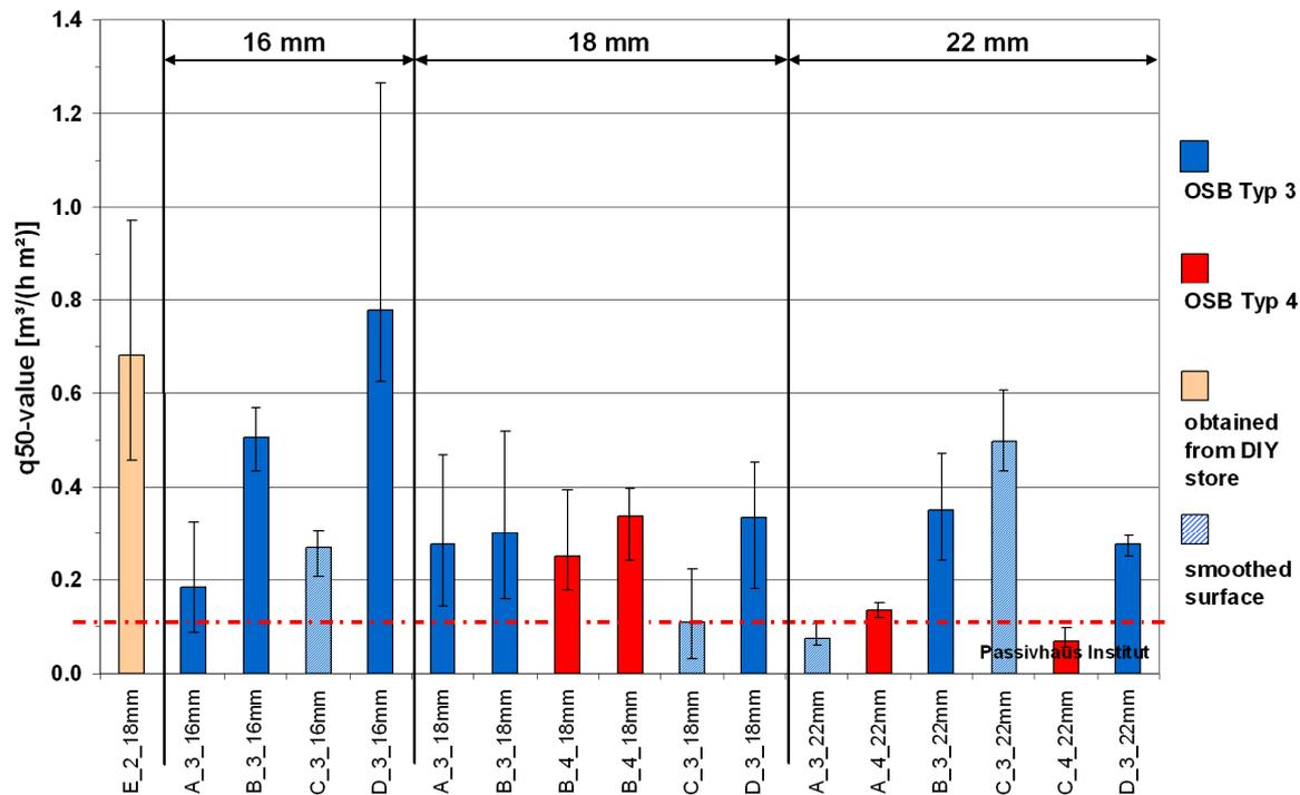
**Figure 2:** Measurement results for airtightness ( $q_{50}$ -value) of "OSB Type 3" and "OSB Type 4" from four different manufacturers (A...D) sorted according to board thicknesses of 16, 18 and 22 mm. In addition, the result for a board obtained from a DIY store is also shown. The average value from three measurements (bar) and the smallest and largest measured value (line depicted as I) are shown. The target value is  $0.1 \text{ m}^3/(\text{m}^2\text{h})$  (dotted red line).
