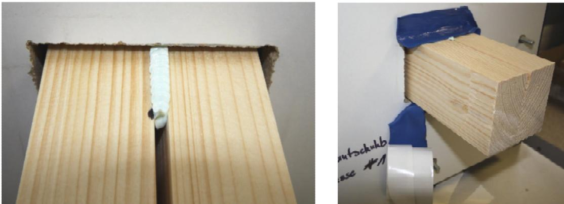
**Figure 19:** Filled in crack with small penetration depth of the sealant (left) and application of the butyl rubber tape (right)
