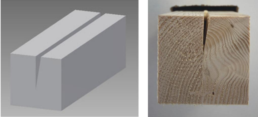
**Figure 12:** 3D model and photograph of the front end of the sample beam (length: 250 mm, edge length: 80 x 80 mm, area of crack: 0.9 cm<sup>2</sup>)
