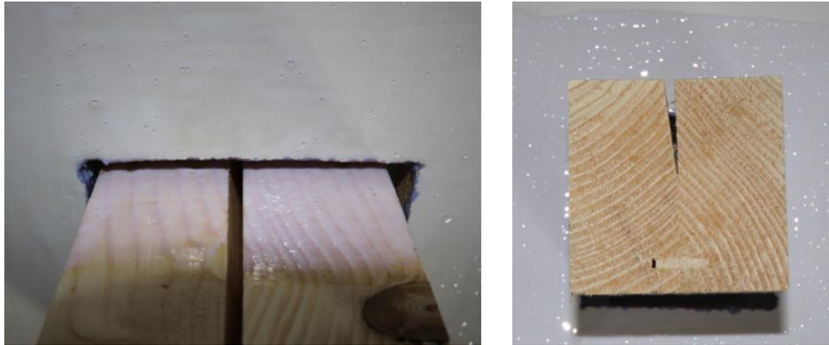
**Figure 16: Beam with adhesive primer prior to application of adhesive tape**
