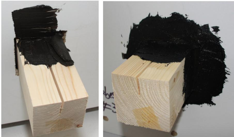
**Figure 30:** Application of the thick bituminous coating for sealing the beam
