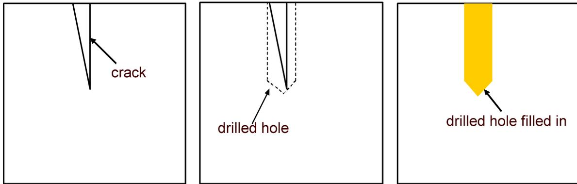
**Figure 24:** Schematic diagram (beam section) of the procedure for the solution with a drilled hole for sealant, with drilling and filling of the crack in the beam. Filling the hole with a wooden dowel is also possible.
