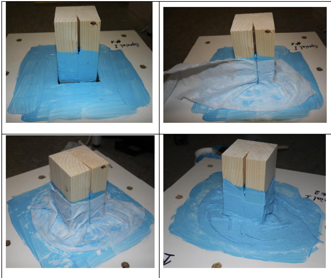
**Figure 20:** Pictures showing the procedure for the "special solution" (above left: initial layer of paste-like compound on the beam and cover; above right: fitting of the material into the gaps and crack; below left: material fitted and pressed on, folds can be seen clearly; below right: second coat of paste-like compound/saturated material)
