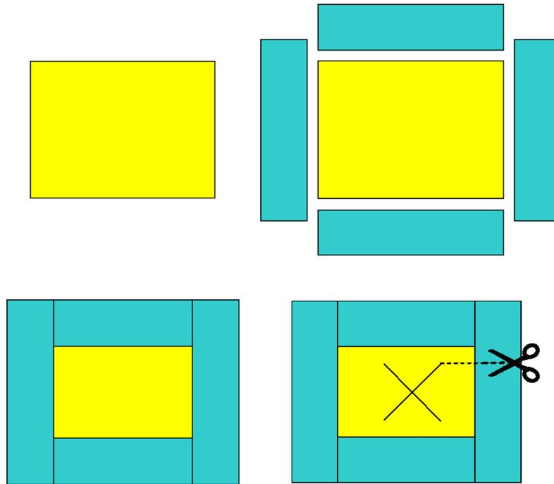
**Figure 26:** Schematic diagram of the work steps for creating a sealing membrane collar (yellow: sheeting, turquoise: adhesive tape). See text for explanations.
