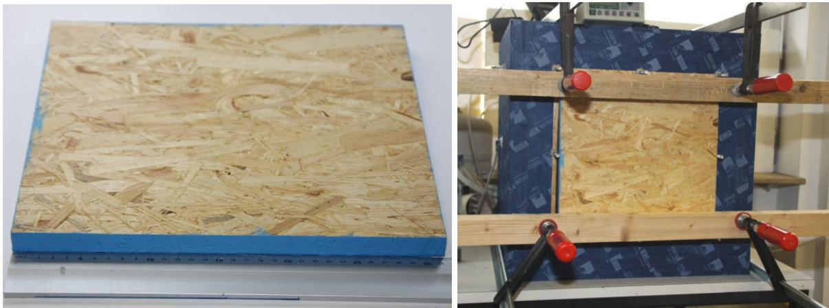
**Figure 36: OSB sample with sealed edge (left) OSB sample attached to the test box using two-by-fours and screw clamps (right)**
