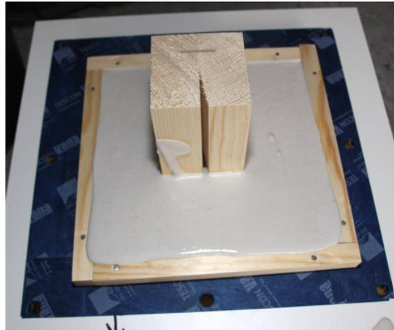
**Figure 28: Horizontal poured gypsum plaster (thin liquid, with wooden frame)**
