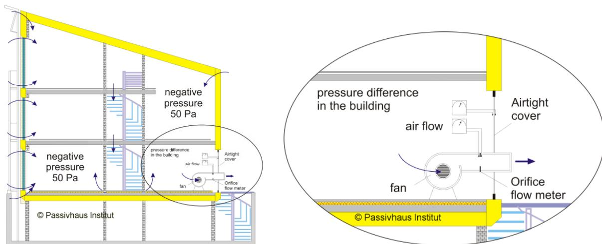
**Figure 5:** Basic test set-up for an airtightness measurement [Peper/Feist/Sariri 1999/2009])
