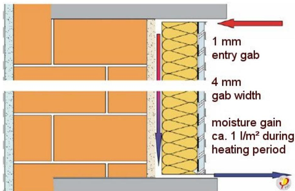
Figure 4: Convective moisture gain with air flow behind interior insulation [Pfluger 2005])
