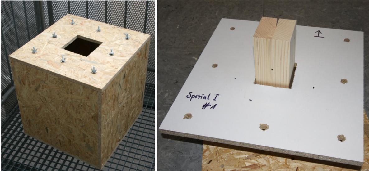
**Figure 11:** Test box with opening and screws for fixing the cover, without adhesive tape covering and without sealing of the cover (left). Cover with penetrating beam, here without sealing, with holes for screws (right).
