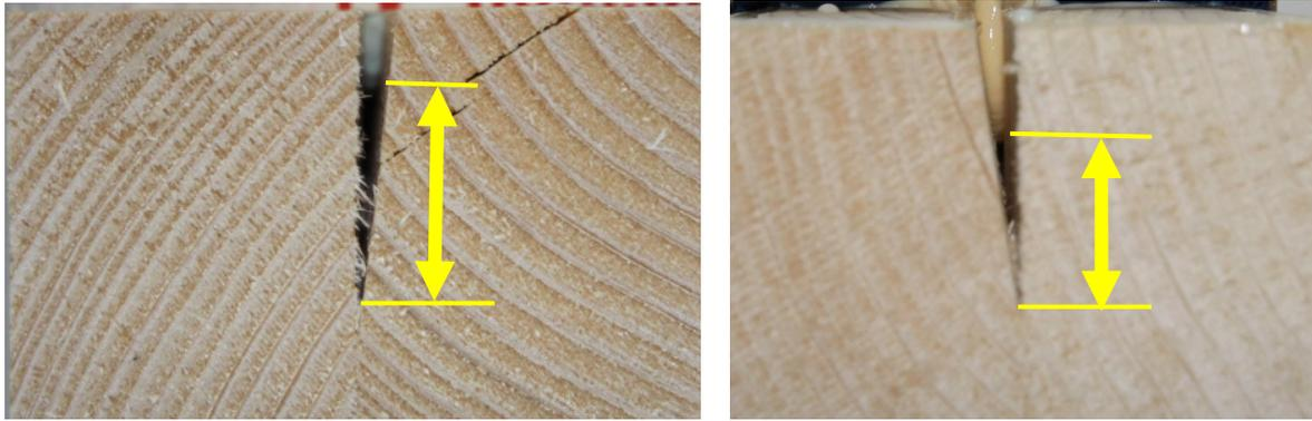
**Figure 17: Penetration depth of the sealant in the crack with the methods AAS I and AAS II. The arrows show the remaining gap.**
