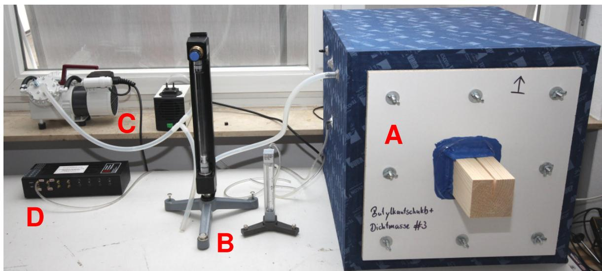
**Figure 10:** Test set-up at the Passive House Institute for the airtightness measurement for beam heads (A: test box with cover and a sealed sample beam; B: variable area flowmeter; C: membrane vacuum pump; D: differential pressure measurement)
