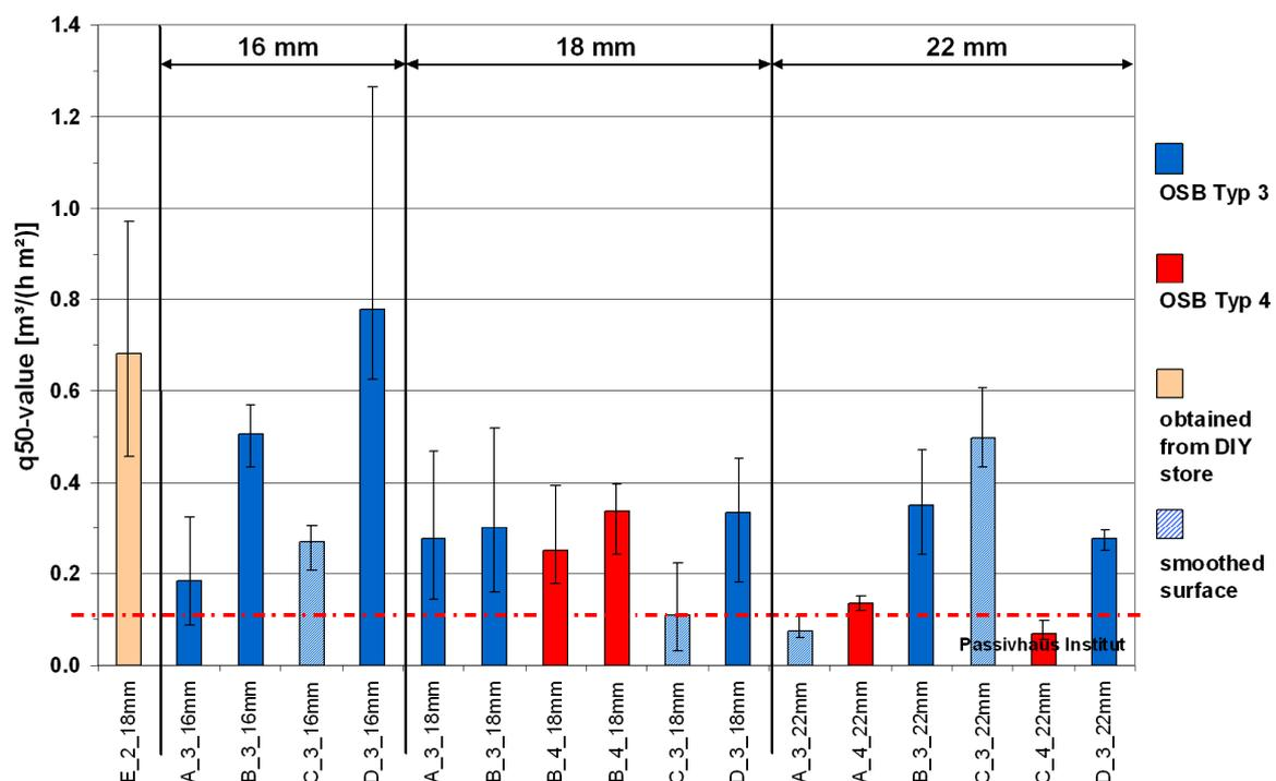
**Figure 37:** Measurement results of airtightness ( $q_{50}$ -value) of Type 3 and Type 4 OSBs from four manufacturers (A...D) sorted in order of board thickness with 16, 18 and 22 mm. The result for a board obtained from a DIY store is also shown additionally. The mean value of three measurements (bar) and the minimum and maximum value (line with I) are shown. The target value is  $0.1 \text{ m}^3/(\text{m}^2\text{h})$  (red dotted line-).
