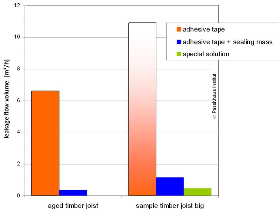
**Figure 34:** Leakage volume flow at a differential pressure of 50 Pa for the "real" beam and the "large" sample beam with the sealing using the methods adhesive tape only (without filling of cracks), adhesive tape + sealant and the "special solution" (pure acrylate dispersion)
