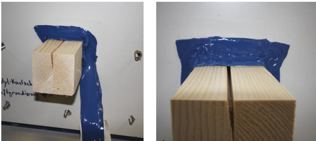
**Figure 18:** Procedure with butyl rubber tape (left: application in one piece; right: very small penetration depth of the elastic adhesive material into the crack)
