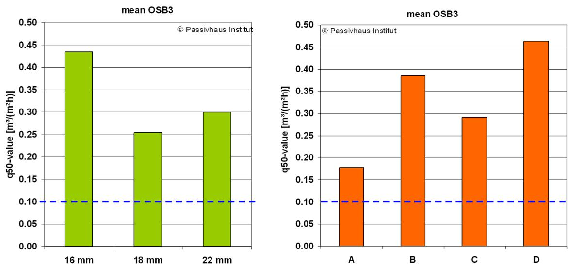
**Figure 38:** Average values of the measured values for Type 3 OSBs shown in Figure 37, according to board thickness (left) and manufacturer (right); averaged with the board from the DIY store; blue line target value  $q_{50} = 0.1 \text{ m}^3/(\text{m}^2\text{h})$ .
