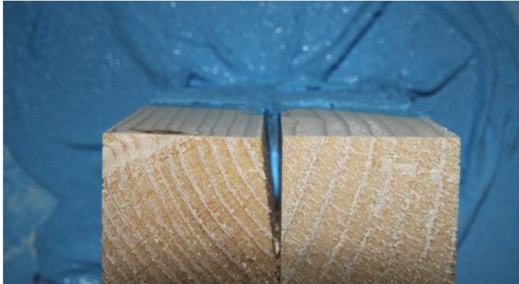
**Figure 21: Crack completely filled with compound**
