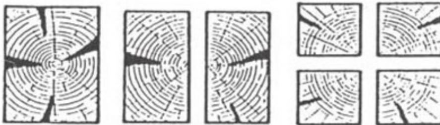
**Figure 9: Course of dry cracks with different types of wood cuts (left: solid wood beam; centre: half beam; right: quartered beam) (Source: [GDHeV])**
