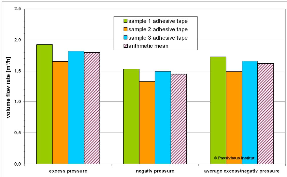
**Figure 15: Measurement results for sealing using adhesive tape at excess and negative pressure for each of the 3 samples, and the arithmetic mean values**
